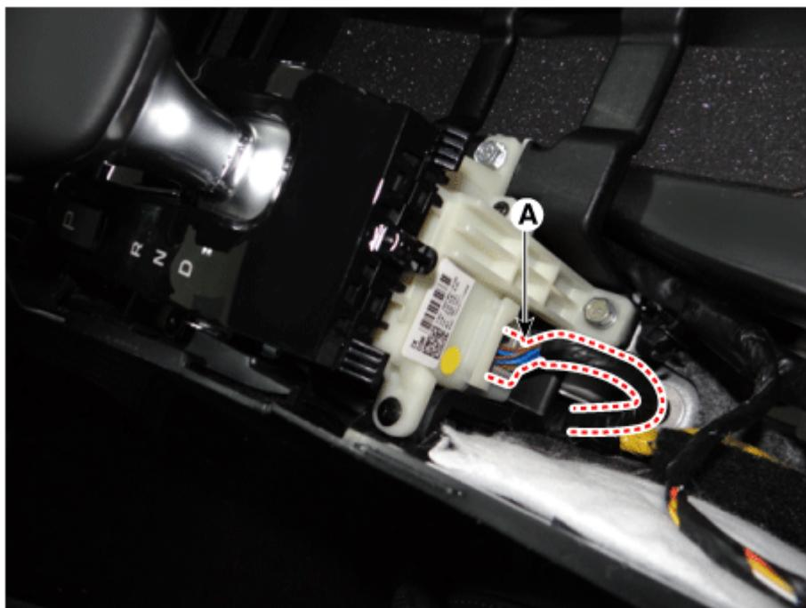
3. Loosen the E-shifter mounting screws (A).
