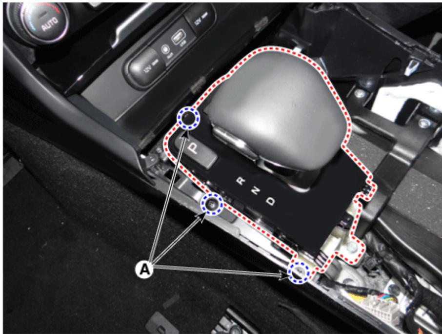
4. Loosen the E-shifter mounting bolts (A).
